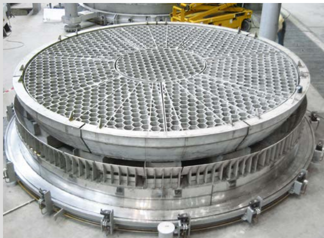
▲ Annealing base for nitrogen and hydrogen annealing with honeycomb grating and set of confusor / difusor parts made from heat-resistant material
