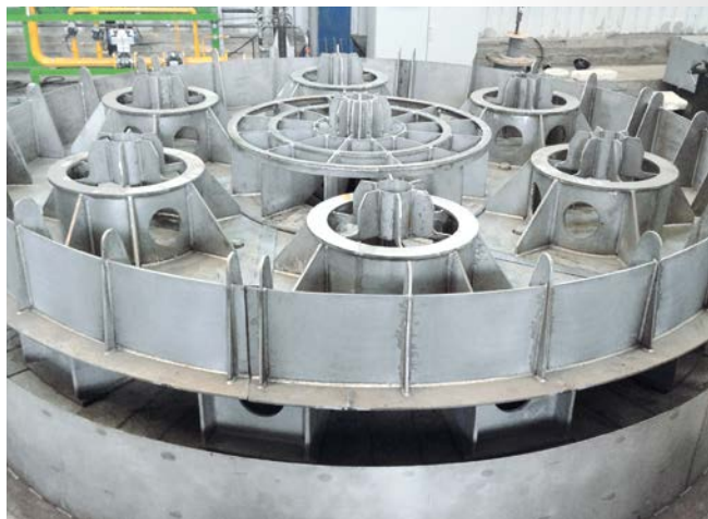
▲ Base designed with FEM strength modelling, equipped with fixed charging stations for extremely high stability
