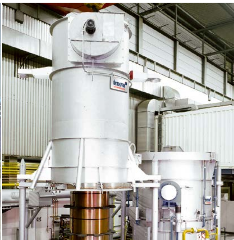
▼ HPH® Bell-type Annealing Plant plant for bright annealing CuZn coils
