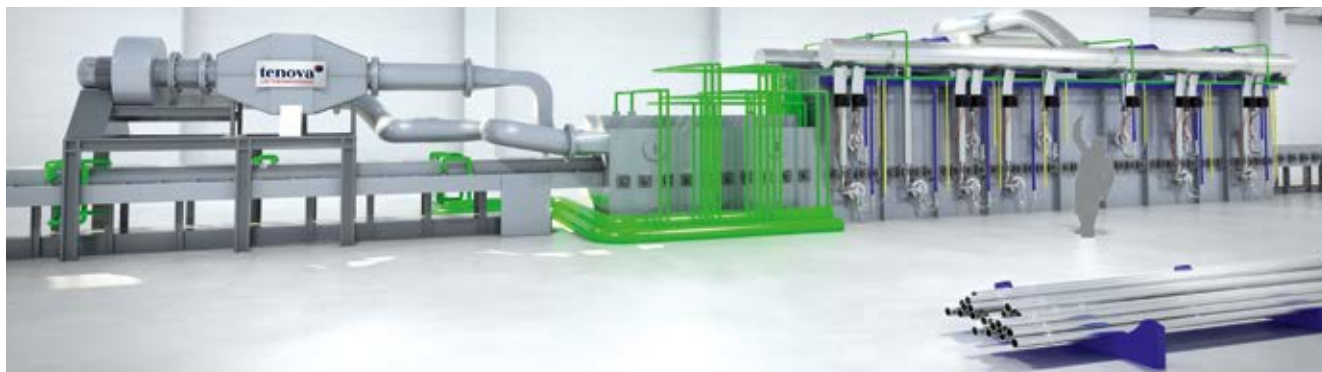
▲ 3-D illustration of a Roller Hearth Furnace for high-alloy steel tubes with hydrogen jet cooling
