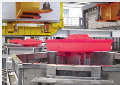
▼ Hardening tables operating in-line with the forging press 与锻压机同步操作的淬火台
