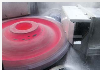
▼ Dedicated nozzle system spraying water onto the wheel 车轮喷水淬火专用喷嘴系统
