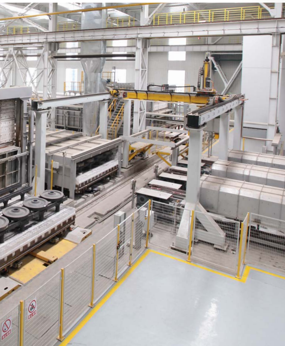
▼ Hardening tables operating in-line with the forging press 与锻压机同步操作的淬火台
