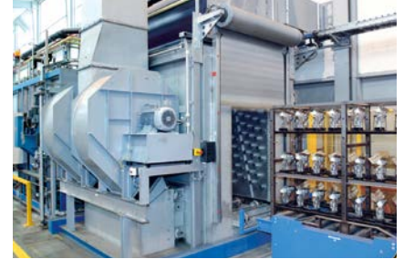
▲ Tenova LOI Thermprocess AirQuenchSystem AQS for structural components
