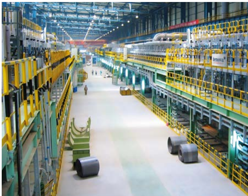
▲ Tenova LOI Thermprocess FCL® for Flattening and Coating of GO silicon steel strip
