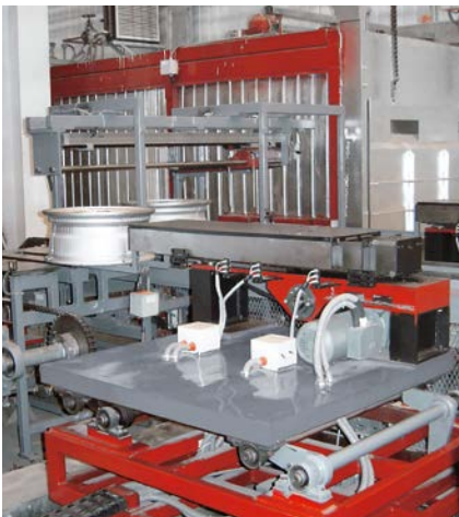
▲ Tenova LOI Thermprocess multi-lane chain conveyor furnace with single-part quenching
