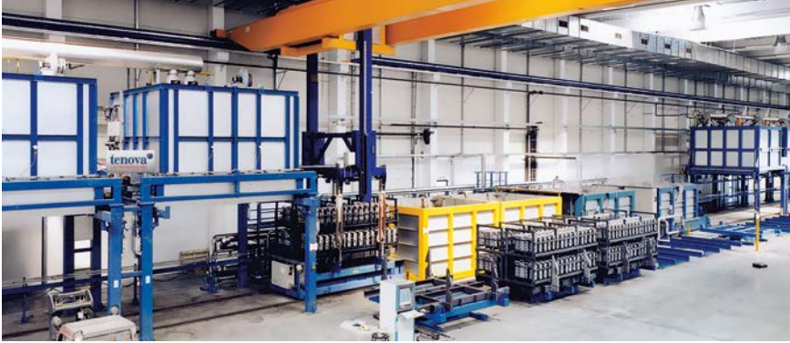
▲ Tenova LOI Thermprocess AirQuenchSystem AQS for structural components
