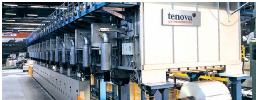
▲ Tenova LOI Thermprocess Single-Coil Annealing Line SCL for aluminium strip
