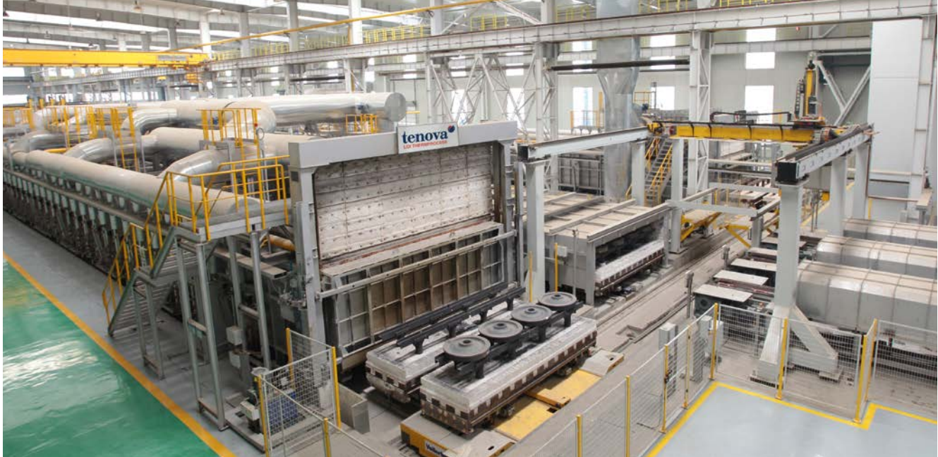
▲ Tenova LOI Thermprocess continuous heat treatment line for high-speed railway wheels
