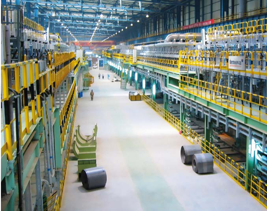
▲ Tenova LOI Thermprocess Flattening and Coating Line FCL for GO silicon steel strip
