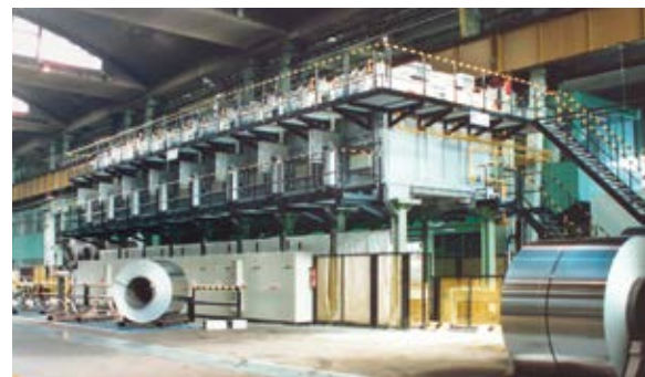
▲ Tenova LOI Thermprocess Final Annealing Line FAL for heat treatment of aluminium foil rolls
