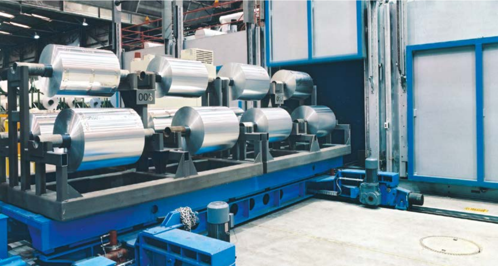
▲ Multi-chamber annealing furnace plant for annealing of foil coils FAL. ▼ 用于铝箔卷材退火的多室式退火炉FAL
