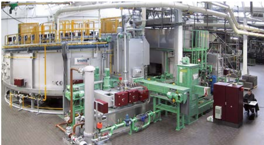
▲ Tenova LOI Thermprocess Rotary Hearth Furnace with zone separation for gas carburizing of gear parts and Q&T steels.
