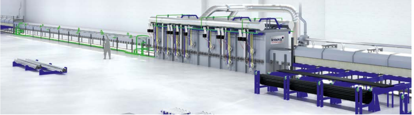
▲ 3-D illustration of a Roller Hearth Furnace for carbon steel tubes with radiant cooling
